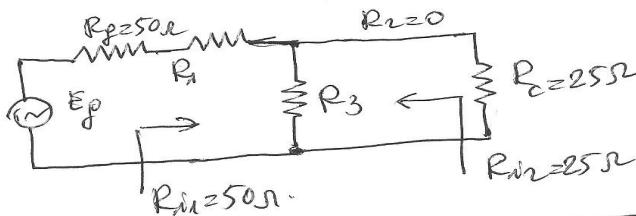
$$R_3 = \frac{2\sqrt{k}}{k-1} \sqrt{R_{11} R_{12}}$$
