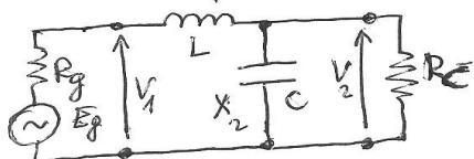
$$\begin{aligned} X_1 &= X_L = Q_p R_g = 2,236 \cdot 50 = 111,8 \Omega \\ X_L &= 2\pi f L \\ L &= \frac{X_L}{2\pi f} = \frac{111,8}{6,28 \cdot 10^6} = 1,82 \cdot 10^{-5} \text{ H} = 1,82 \mu\text{H} \end{aligned}$$
