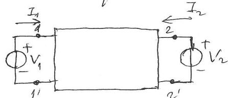
$$Y_{11} = \left. \frac{I_1}{V_1} \right|_{V_2=0}$$
