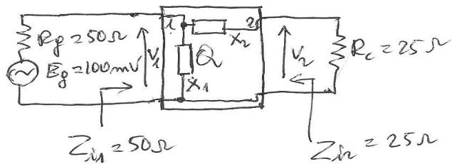
$$V_1 = \frac{E_g Z_m}{Z_m + R_p} = \frac{E_g \cdot 50}{50 + 50} = \frac{E_g}{2} = 50 \text{ mV}$$
