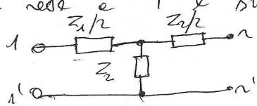
$$\begin{aligned} Z_{11} = Z_{22} &= \sqrt{\frac{z_1^2}{4} + \frac{z_2^2}{4} + \frac{z_1 z_2}{2}} \\ &= \sqrt{\frac{z_1 z_2 + z_1^2}{4}} \end{aligned}$$
