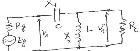
$$\begin{aligned} X_1 &= X_C = Q_p R_g = 111,8 \Omega \\ X_1 &= \frac{1}{2\pi f C} ; \quad C = \frac{1}{2\pi f X_C} = \\ &= \frac{1}{6,28 \cdot 10^6 \cdot 111,8} = 1,424 \cdot 10^{-9} \text{ F} = \\ &= 1,424 \text{ nF} \end{aligned}$$
