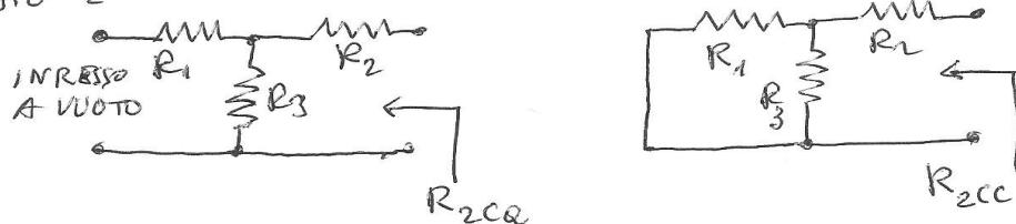
$$R_{2cc} = R_2 + R_1 // R_3 =$$
