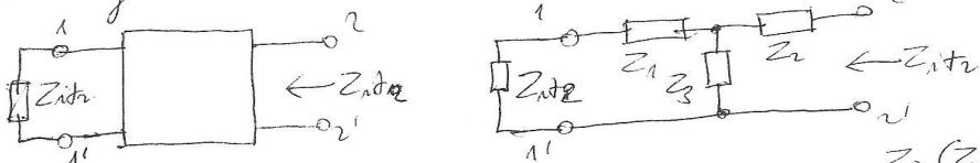
$$Z_{load} = Z_1 + Z_3 / (Z_2 + Z_{load}) = Z_1 + \frac{Z_3 (Z_1 + Z_{load})}{Z_2 + Z_1 + Z_{load}}$$
