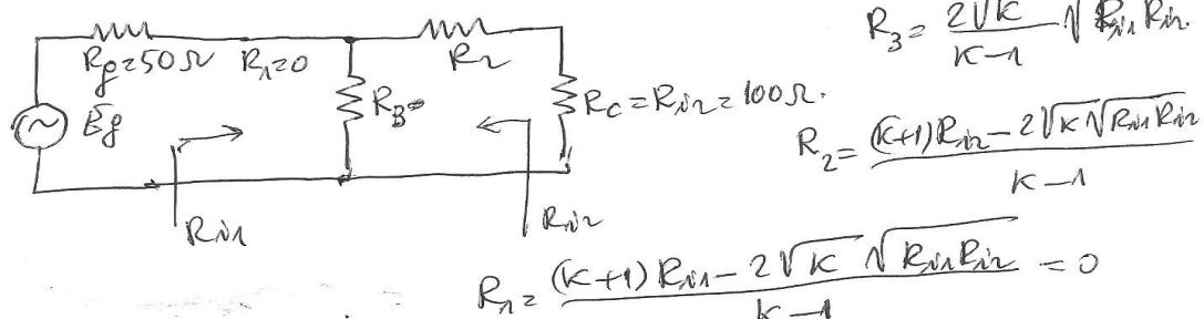
$$(k+1)R_{in} = 2\sqrt{k}\sqrt{R_{in} R_{in}} \quad \text{se } R_1 = 0$$
