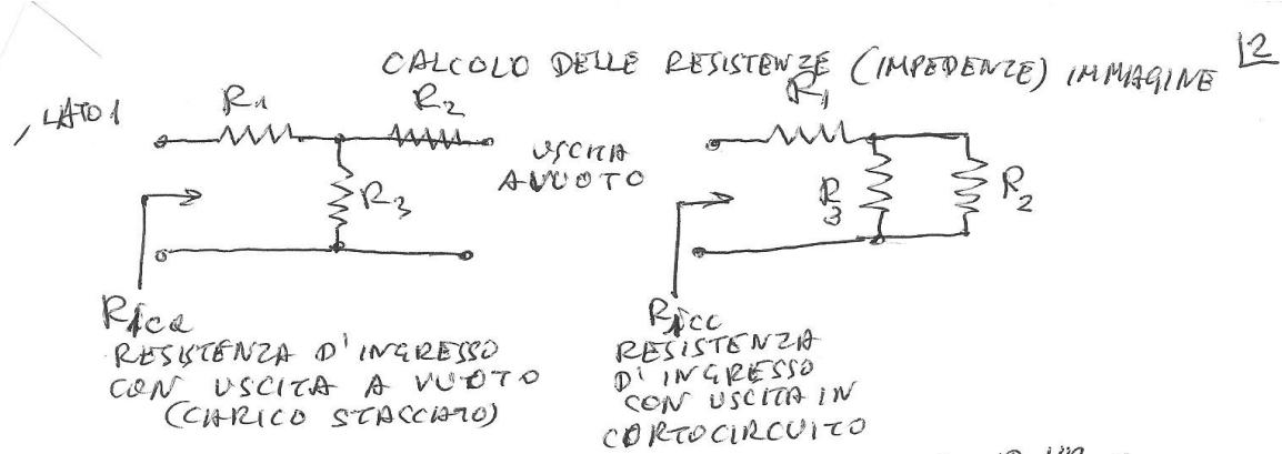
$R_{1'i} = \sqrt{R_{1ce} \cdot R_{1cc}} = \sqrt{(R_1 + R_3)(R_1 + \frac{R_2 R_3}{R_2 + R_3})} =$
