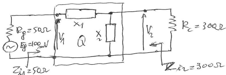
$$V_A = \frac{E_f Z_{in}}{Z_m + R_g} = \frac{E_f \cdot 50}{50 + 50} = \frac{E_f}{2} = 50 \text{ mV}$$
