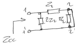
$$Z_{ca} = 2Z_2 / (Z_1 + 2Z_2) = \frac{2Z_2 (Z_1 + 2Z_2)}{2Z_2 + Z_1 + 2Z_2} = \frac{2Z_2 (Z_1 + 2Z_2)}{Z_1 + 4Z_2}$$
